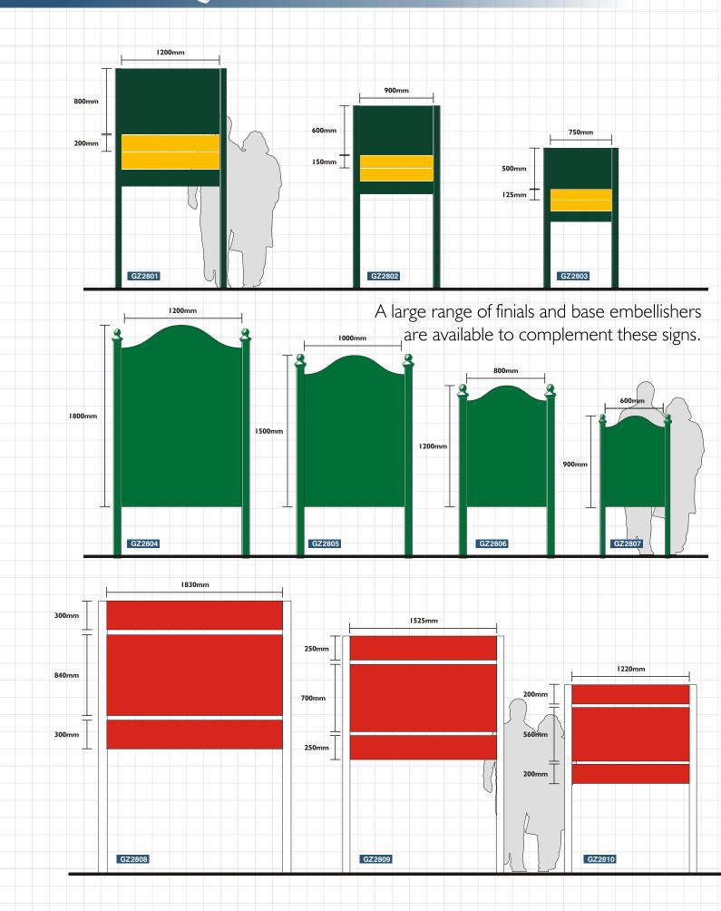
'Plaza' allows you to include a wide variety of shaped or angled tops with the option of fitting posts inboard or outside the sign assembly.
