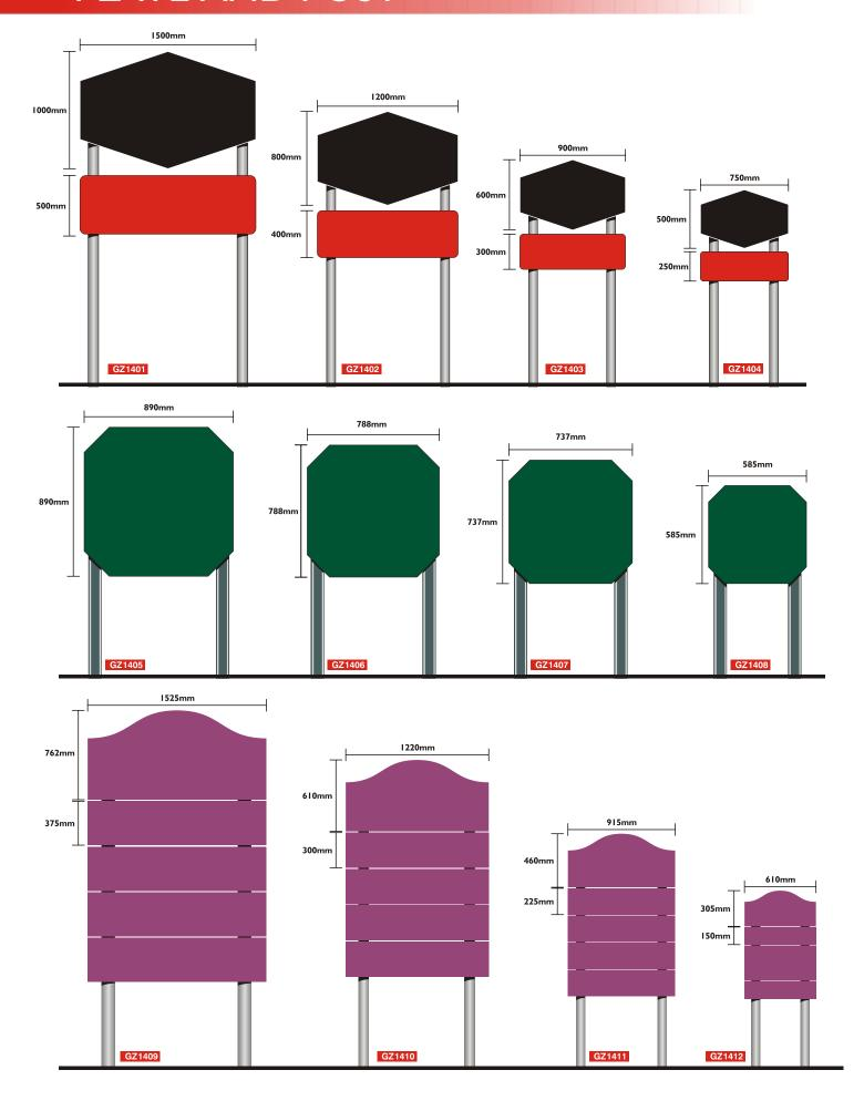
Using the plate and channel system almost any size of sign blank can be produced including large or outsize assemblies.
